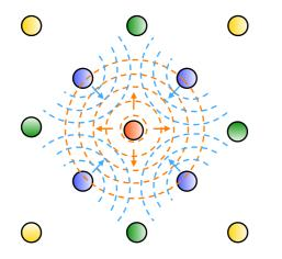
The outgoing spherical wave is scattered by the (coloumb) potentials of neighbor atoms causing interference with itself. The absorbing atom serves both as the source of the photoelectron and the detector. In other words, the XAFS signal reflects the local neighborhood about the absorbing atom.
