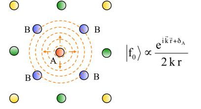
For a s-state core level, an outgoing spherical wave moves out from the absorbing atom.
