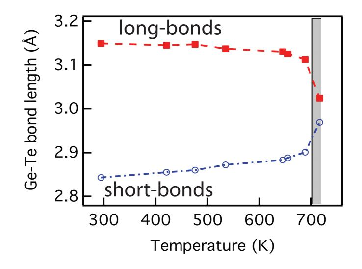
Neutron powder diffraction shows long- and short-bonds calculated from average structure become equal at T<sub>c</sub>
